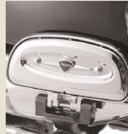
PILLION FOOTBOARD COVERS - CHROME A9738077 Shown fitted with Pillion Footboard Embellishers A9938096
